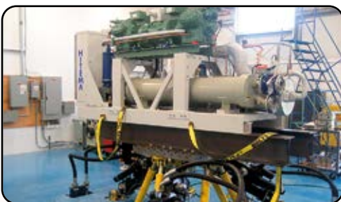
* Seismic test, installed in Canada, 300 kW
